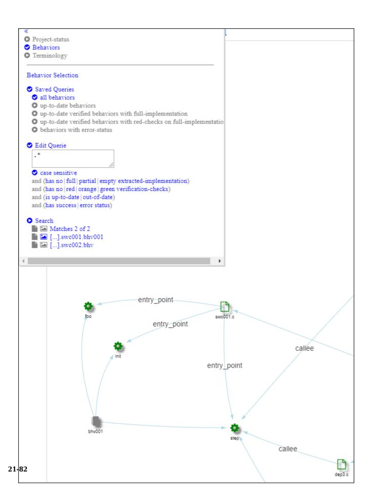
In this example, you see that the software component with internal behavior bhv001 has three runnables implemented through the entry-point functions foo, init, and step. All three entry-point functions are defined in the file swc001.c.
