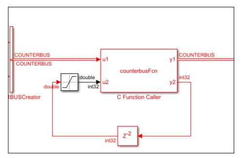
**2** On the **Signal Attributes** tab, specify a minimum and maximum value for the Saturation block output.
