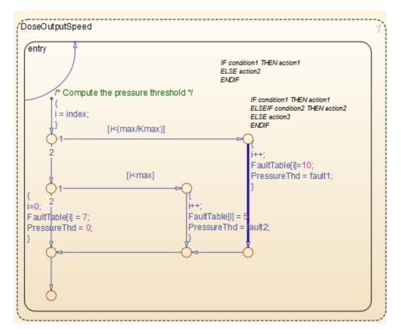
One possible solution to avoid the orange **Out of bounds array index** violation is to constrain the input variable index. Use a Saturation block before the Stateflow chart to limit index between zero to 100. After running the analysis on the modified model, the orange check is resolved.
