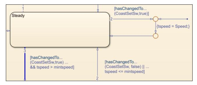
Note the design flaw. The condition for outgoing transition 3 cannot be true without the condition for outgoing transition 2 also being true. Therefore, transition 3, which executes later, is never reached. This design flaw in the chart translates to the unreachable if block in the generated code.
