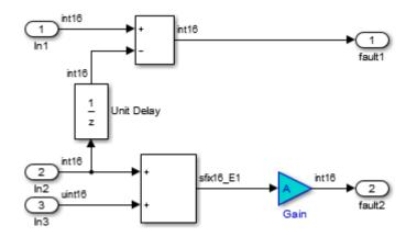
One possible solution to avoid the orange **Overflow** error is to constrain the value of the signal in\_battery\_info that is fed to the Sum block.
